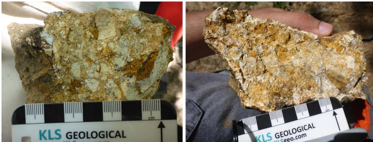
*Figure 3 - Hydrothermal / tectonic breccia on the contacts of rhyolitic dykes at Belopoltsi target*
